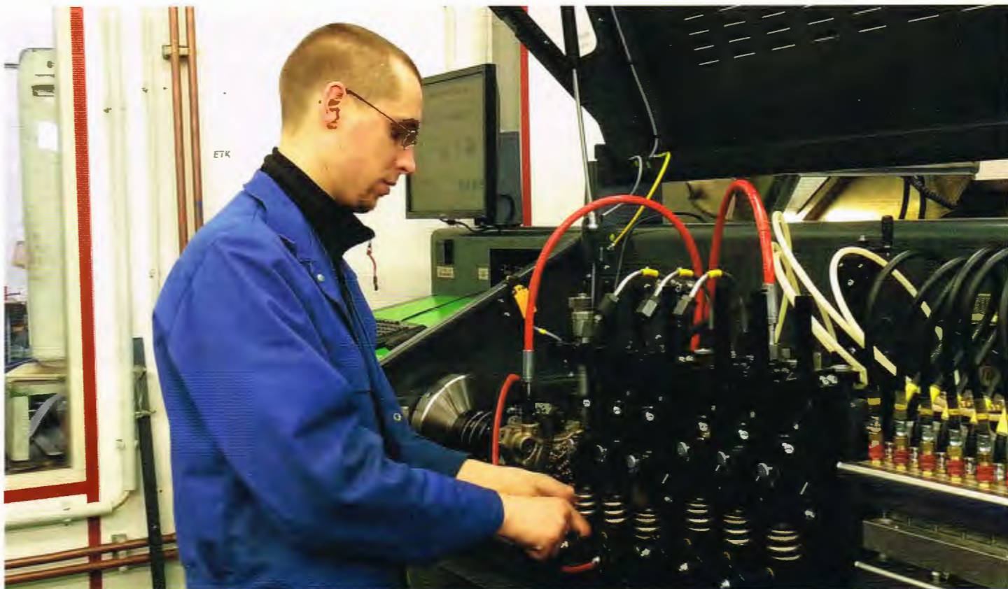
The diesel centre is equipped with high-tech test systems for remanufacturing of injectors.
