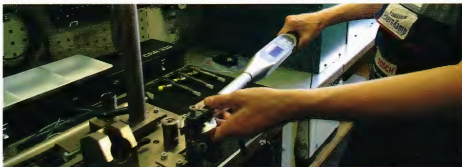
This computer-controlled torque wrench is used for repair stage 3 (currently highest stage) of the last generation of Bosch injectors.
